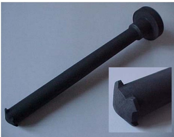
Fig. 1 Photograph of the thermometer well of the Co_4N8_long cell with an enlargement of the bottom, specially designed to allow a safe vertical introduction into the crucible
